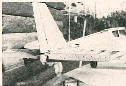
Picture #9 Bottom view showing elevator horn and pushrod. Horns are from the same "Midwest Nylon Builders' Accessory Kit C-5" as the brain bell-cranks in the fuselage. Notice the dowel stabilizer keys to prevent shifting in flight. These are essential. Details of control surface travel are given in sketch.
