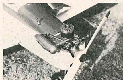
Picture #9 Bottom view showing elevator horn and pushrod. Horns are from the same "Midwest Nylon Builders' Accessory Kit C-5" as the brain bell-cranks in the fuselage. Notice the dowel stabilizer keys to prevent shifting in flight. These are essential. Details of control surface travel are given in sketch.
