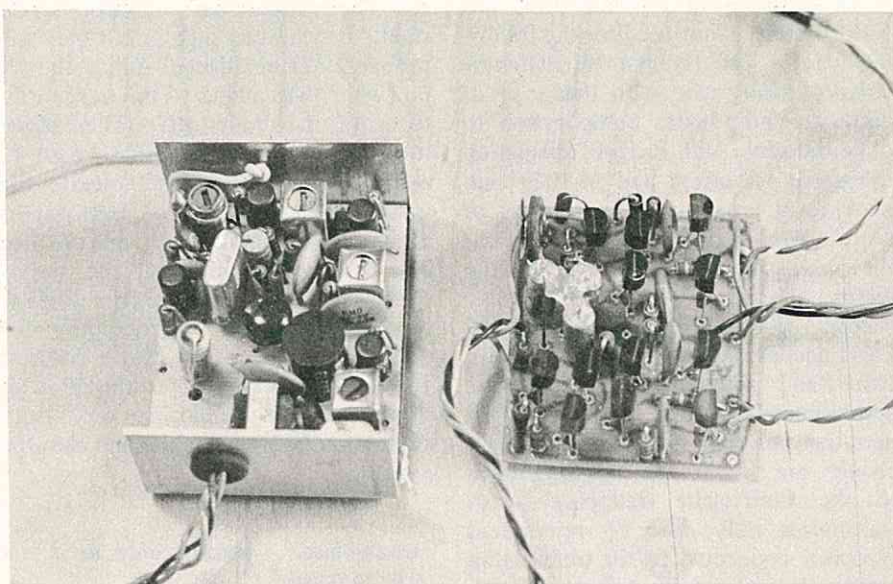
FIGURE 10: Converted Controlaire SH-100 receiver and completed decoder.
