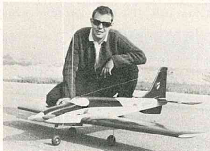
Poldo Pergher and Andromeda M-31, his latest original. Span 60", 6¼ lbs., ST 60 with Kavan carb., Micro Avionics. Extra fin to give smooth knife-edge flying. Poldo, active RC writer.
