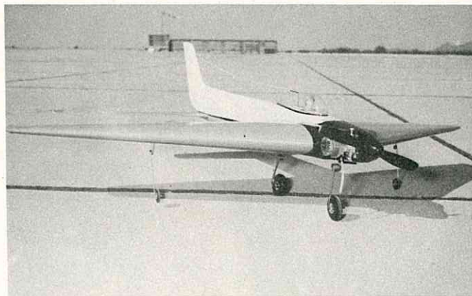
"Trigon" was original pattern stunt ship by Dennis Kohlman of Phoenix ARCS. Featured tandem gear, outriggers and foam delta wing. Impressive performer.
