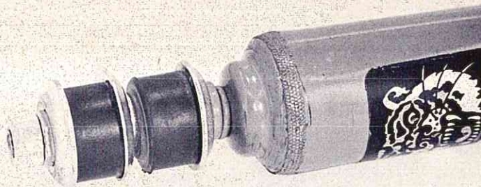
Close-up of front end of shock absorber. Metal "cup" seat between two rubber shock grommets is not used. Upper and lower metal "cups", rubber grommets, and nut are retained.
